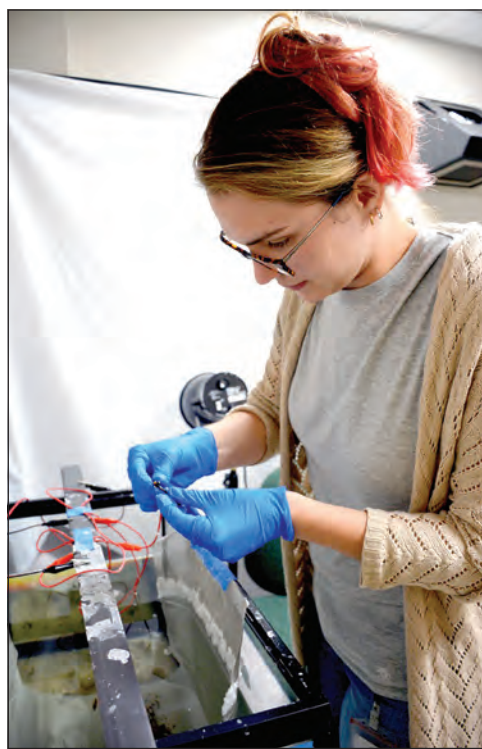
Collections Assistant Deanna de Boer examines a square nail in the electrolysis set up.
