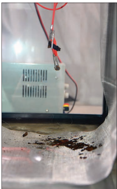
Square nail and nail head suspended in the tank, with corrosion on base.
